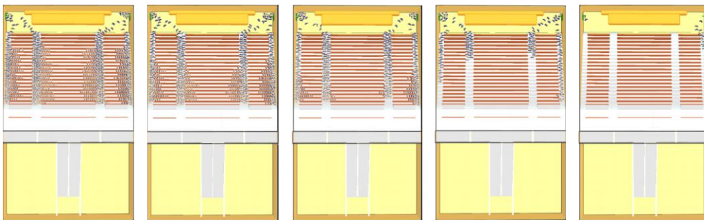
Figure A2.41 FDS+Evac - Positions of persons after 45, 90, 135, 180 and 225 seconds for the 2 nd escape route (S. Schelster)
