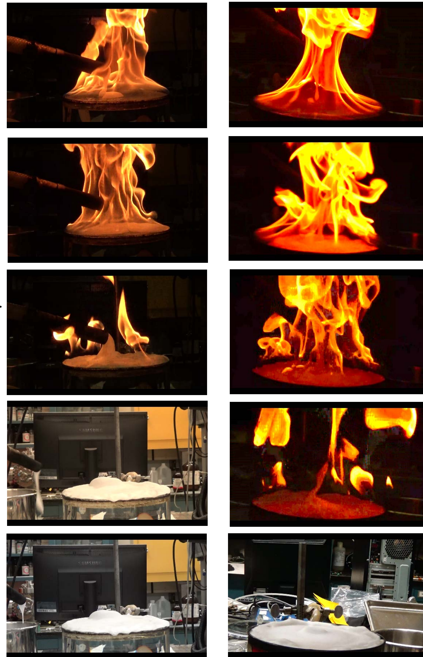
RefAFFF bench scale fire test on heptane pool 502W Formulation fire test on heptane pool
